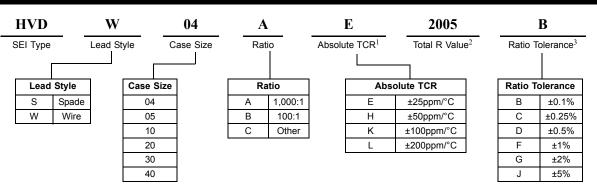
Note 1: TCR Tracking typically <25% of the Absolute TCR to a minimum of 10ppm/°C Note 2: Express value as a four digit number, the first three numbers are the significant value and the forth number is the number of zeros Note 3: The Absolute Tolerance is 5% unless otherwise specified
